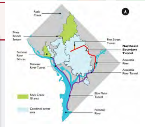
Map of NEBT : Tunnel ends south of RFK Stadium, extends north to Rhode Island Avenue and proceeds to its termination point at the triangle park bordered by Rhode Island Avenue NW, 6th St. NW, and R St. NW. (Source: DC Water, 2017A)
